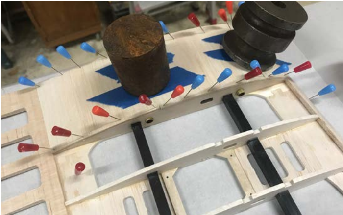
Root area sheeting in place and under weight while the glue dries.
