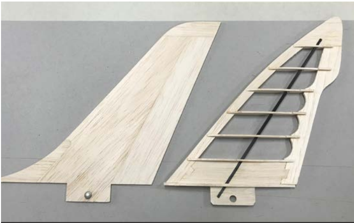
Included sheet fin and the built up option, much better in my opinion.
