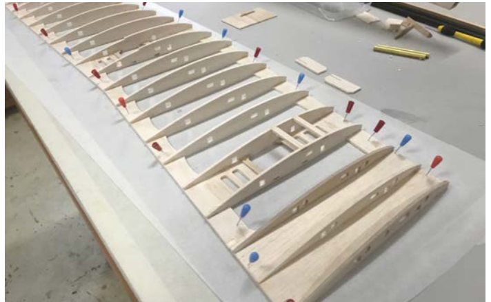
Flat bottom airfoil means the whole wing is built pinned down.
