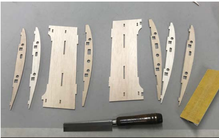
Left and right wing root parts to kick off the wing build.
