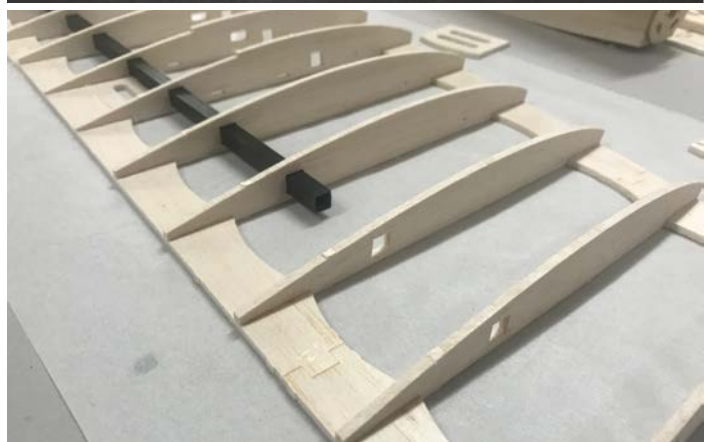
Carbon rod easily slides down every rib for a very clean, snug fit.
