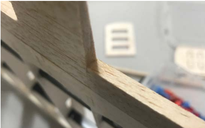
The edge strip has three compound angles for a clean, snug fit.
