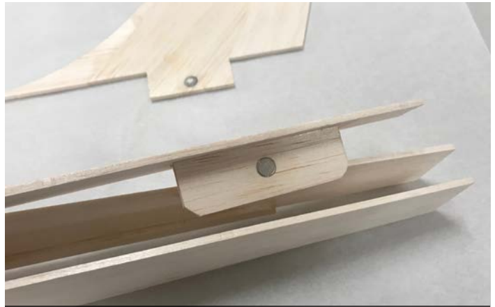
Rare-earth magnets hold the vertical fin in place.
