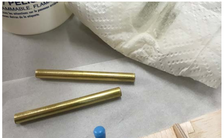
Remember to clean the carbon and brass tubes before gluing.
