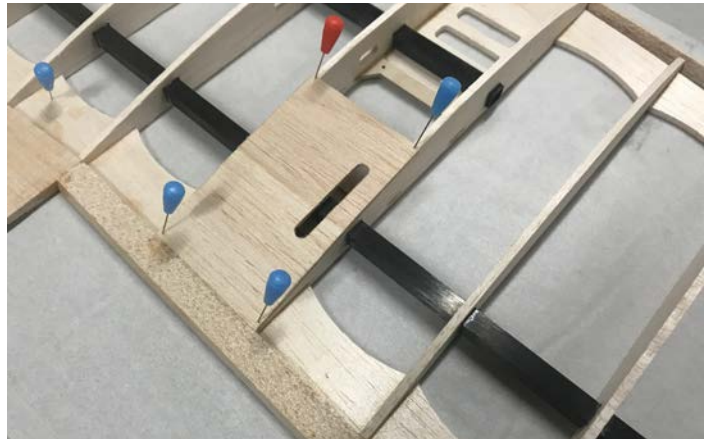
Pushrod exits the top. Hinge is open from the top too, not ideal!
