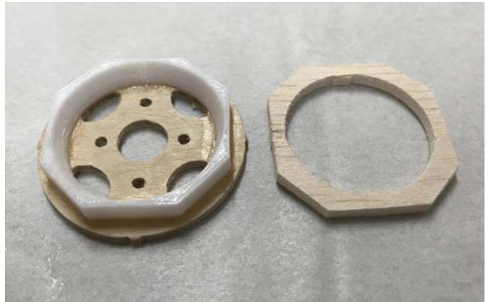
The 3D option allowed a little more clearance for the motor wires.
